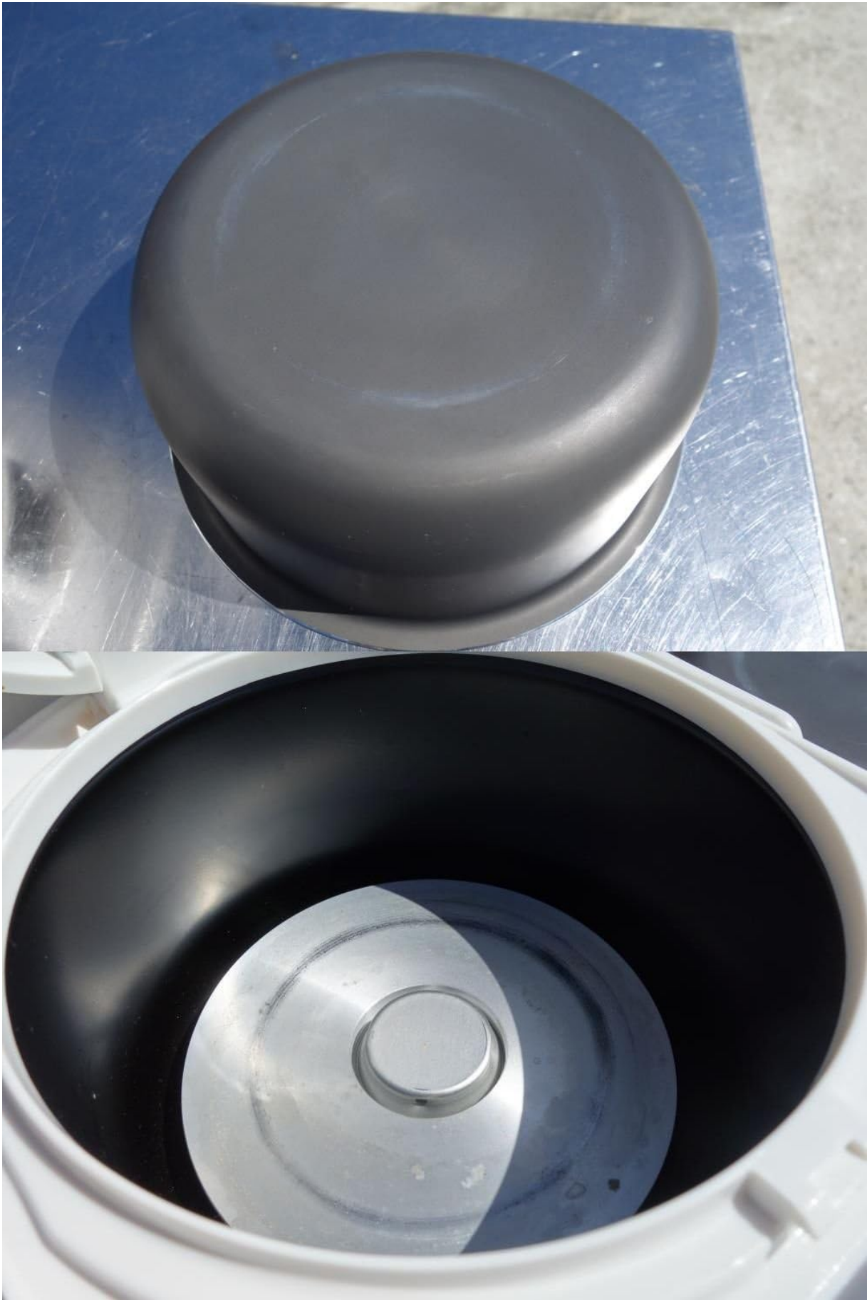
Image 5: The inner pot removed, revealing the heating element inside the main unit.
