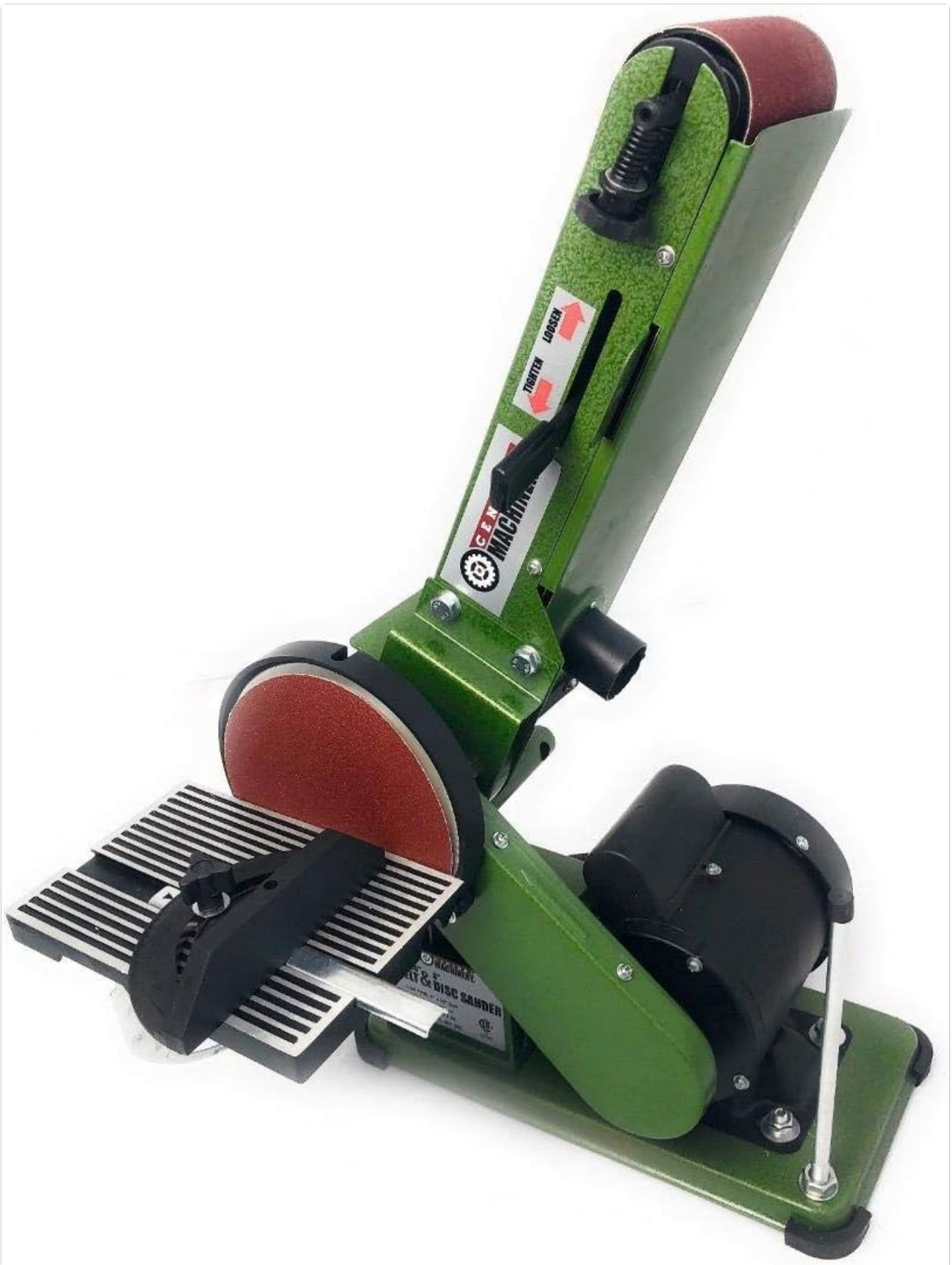
Image 6: The belt sanding arm adjusted to a vertical position, allowing for sanding of longer edges or specific contours.
