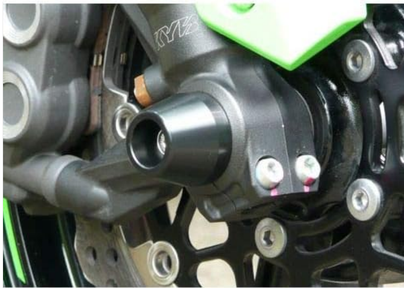
Image: Close-up view of the Aglas Front Axle Slider (cone type, white) securely installed on the front axle of a motorcycle, showing its position relative to the fork leg and brake rotor.
