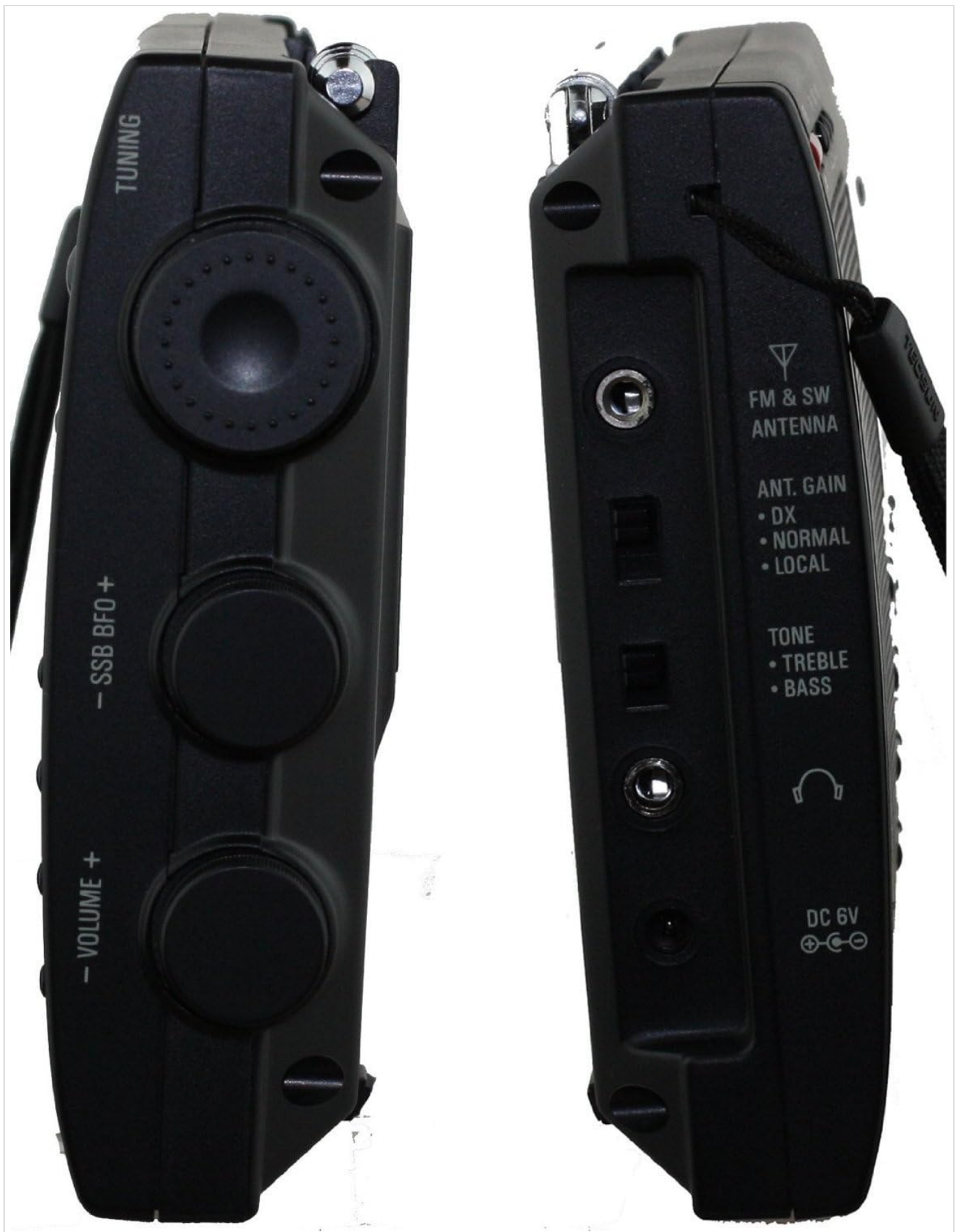
Image: Side view of the TECSUN PL-660 radio. This image shows the rotary tuning knob, the SSB BFO fine-tuning control, and the volume control. Also visible are the external antenna jack, antenna gain switch, tone switch, earphone jack, and DC 6V power input.
