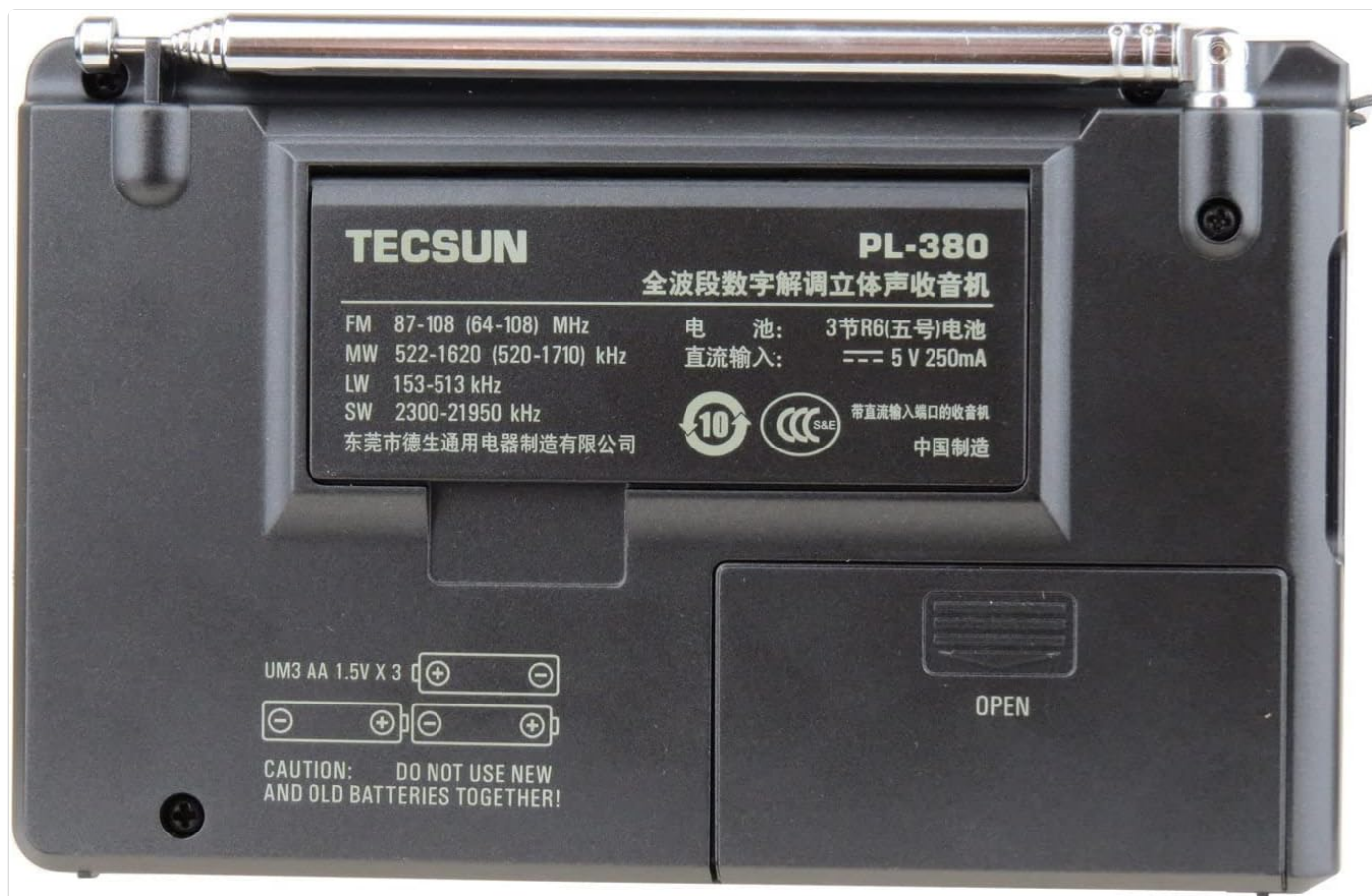
Figure 1: Rear view of the PL-380, highlighting the battery compartment.
