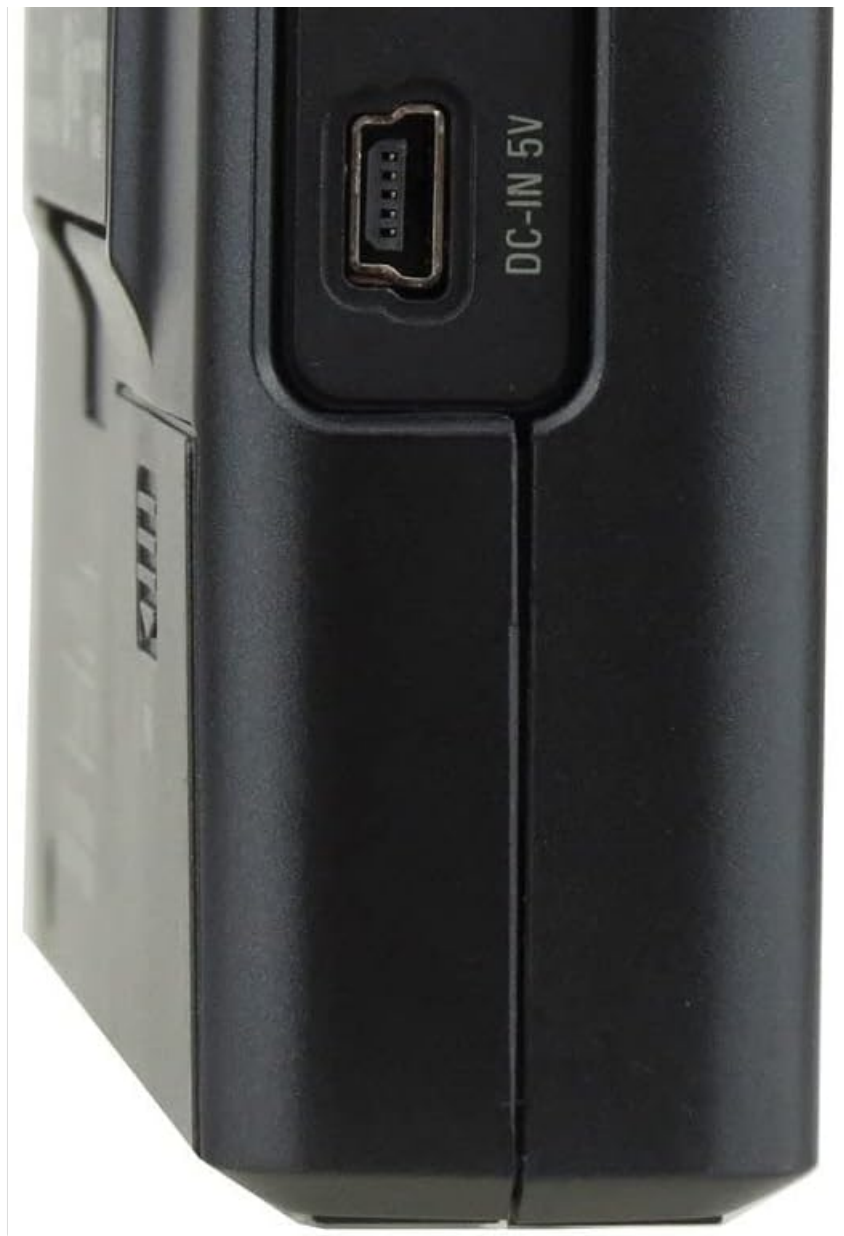
Figure 2: Side view of the PL-380, showing the USB charging port and earphone jack.
