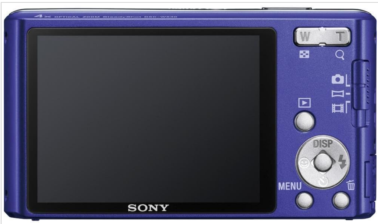
Figure 2: Back view of the Sony Cyber-Shot DSC-W530 camera, highlighting the LCD and control layout.
