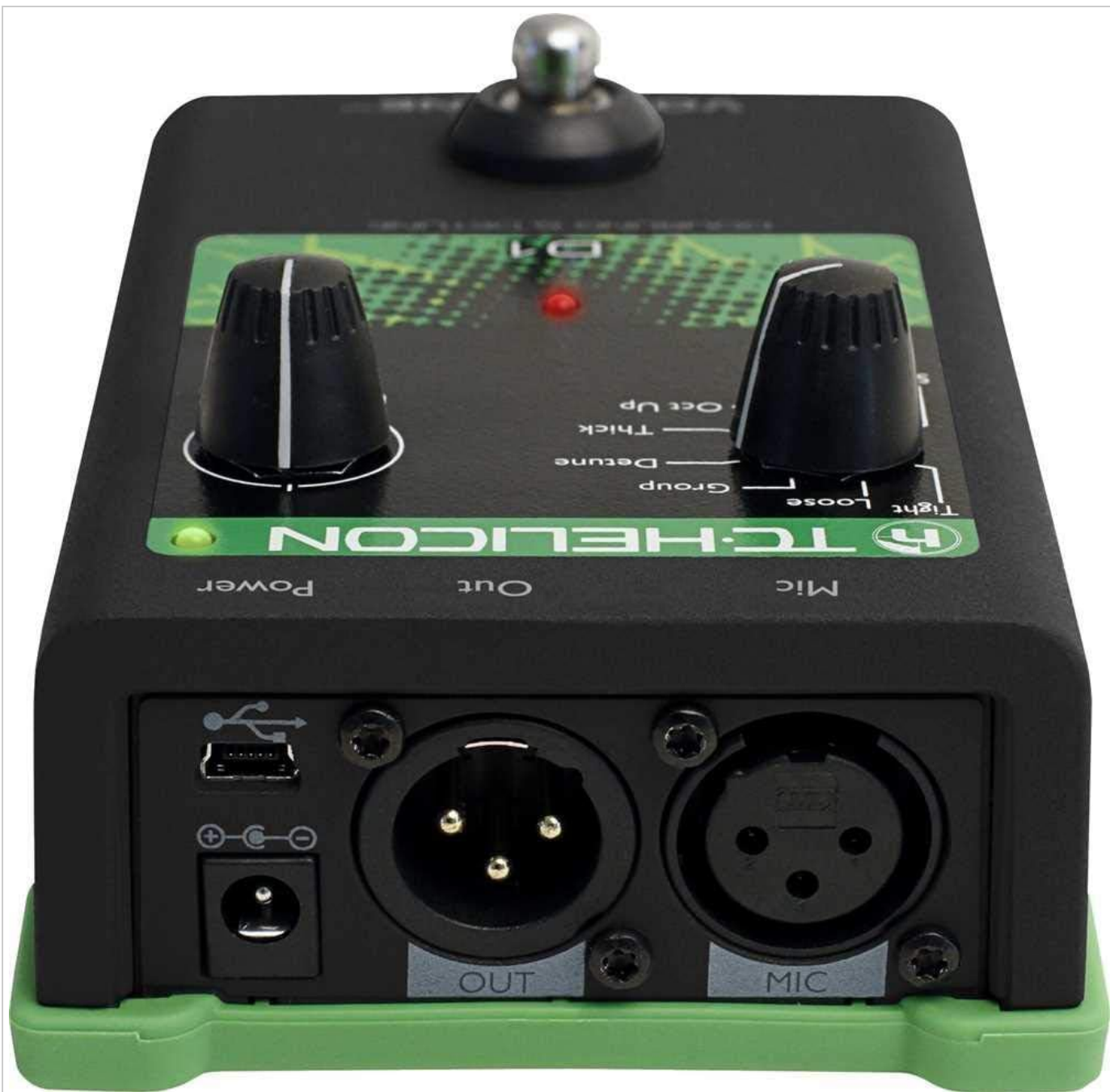
Image: Rear panel connections of the VoiceTone D1, including XLR inputs/outputs and power input.
