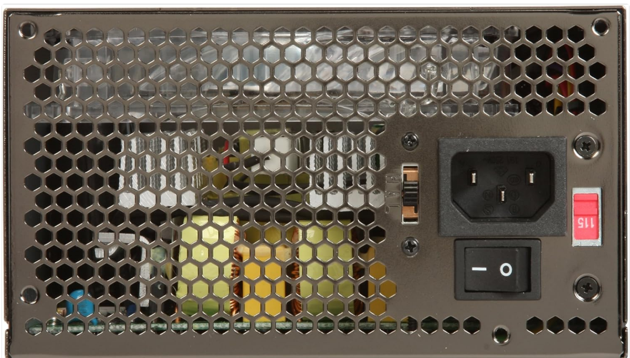
Figure 3.3: Rear panel of the power supply, showing the AC power input, the main power switch, and the red voltage selector switch (115V/230V).
