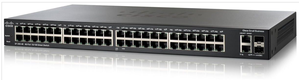
Figure 1: Front panel of the Cisco SF200-48 Smart Switch. It features 48 Fast Ethernet (10/100) ports, arranged in two rows. To the far left, 'System' and 'Reset' indicators are visible. To the far right, two combo Gigabit SFP/mini-GBIC ports are present, labeled G1A and G2. Status LEDs for Link/Act and 100M are located above the Ethernet ports.
