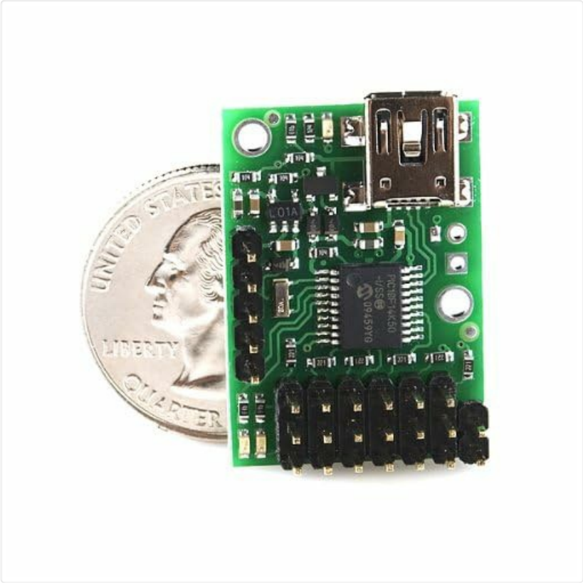
Figure 3: The Micro Maestro shown alongside a US quarter coin, illustrating its compact size.
