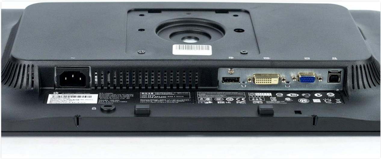
**Figure 3:** Detailed view of the monitor's rear panel, highlighting the power input, DisplayPort, DVI, VGA, and USB ports.
