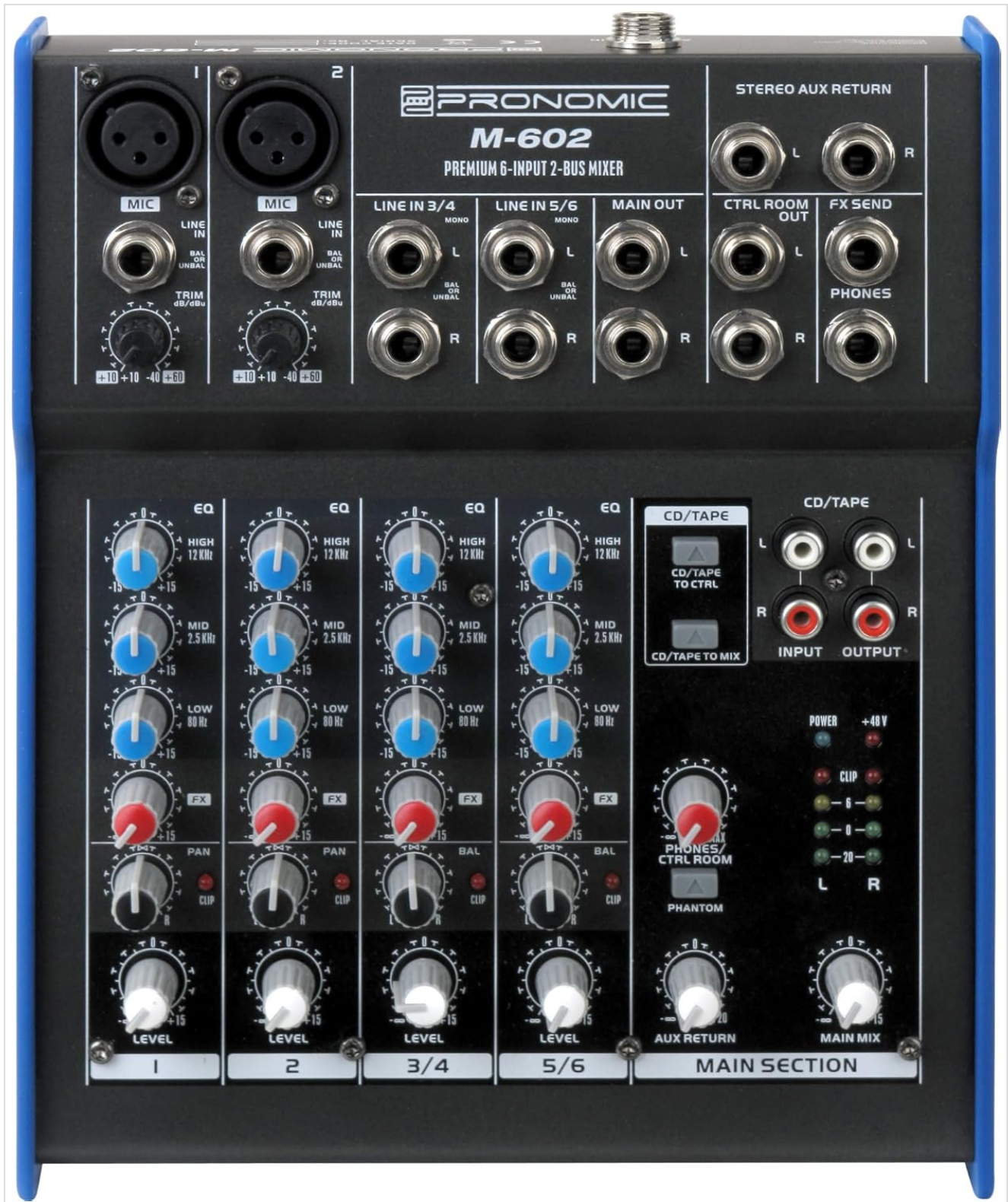
Figure 1: Top-down view of the Pronomic M-602 mixer, illustrating the layout of all controls and input/output jacks. This image displays the two mono channels with XLR/jack inputs, two stereo channels with jack inputs, the main section with CD/Tape I/O, and various output options.
