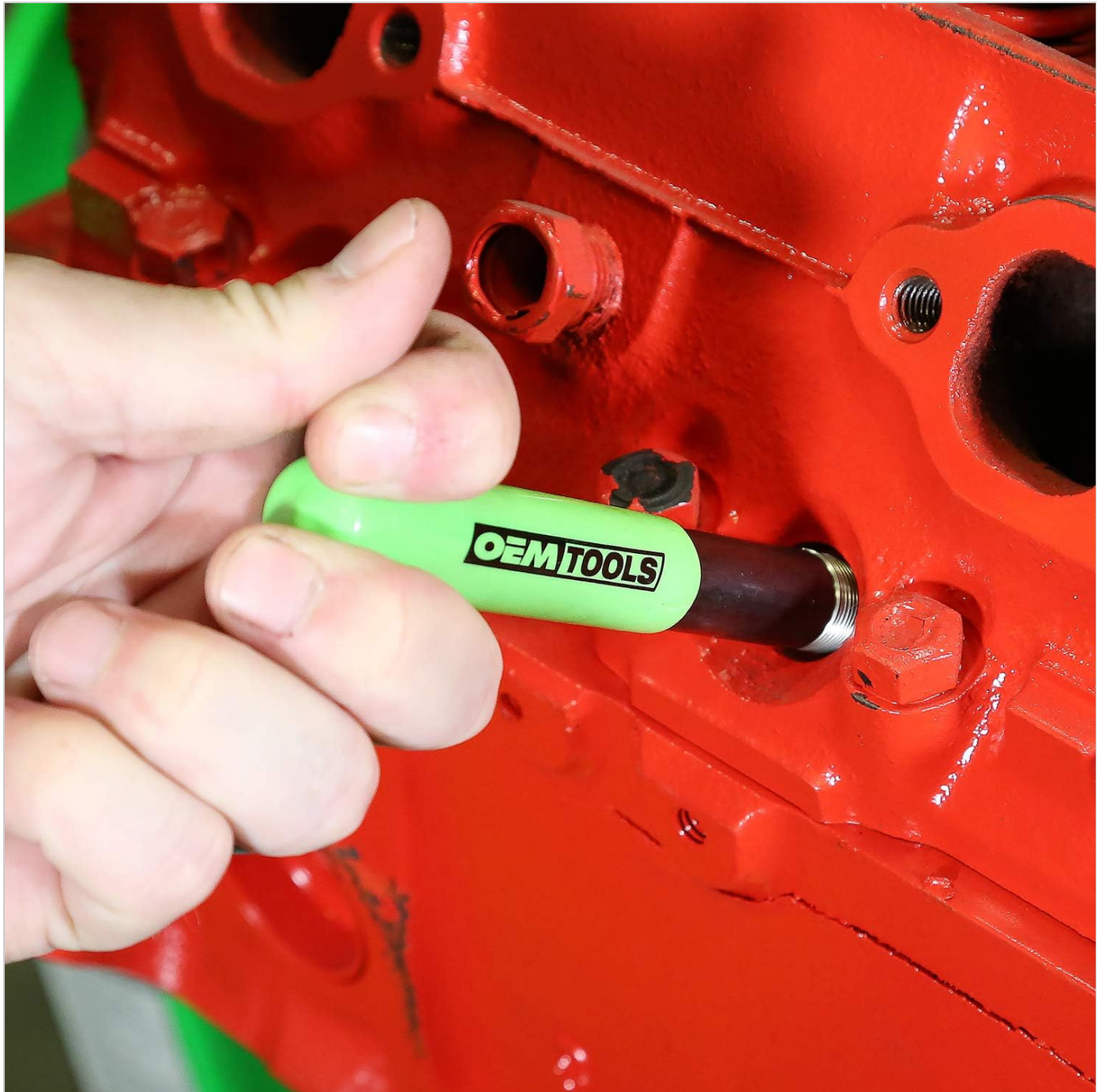
Image: A hand holding the OEMTOOLS thread insert installation tool, threading an insert into a spark plug hole in an engine block.
