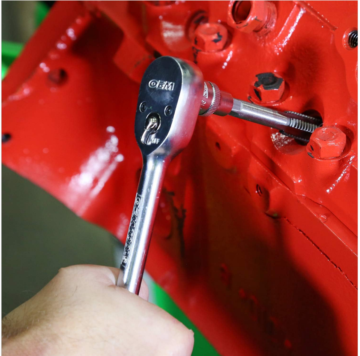
Image: A hand using a ratchet and socket to turn the OEMTOOLS M14-1.25 tap into a spark plug hole, rethreading the damaged area.
