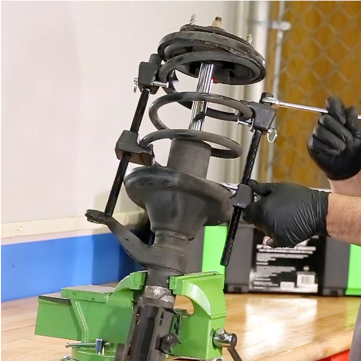
Image 5.2: Spring compressor clamps securely attached to the strut spring.
