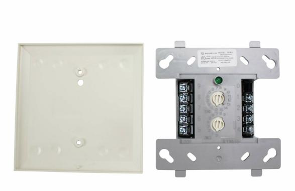
Figure 3: Internal view of the FRM-1 module, revealing the screw terminals for loop and address connections, and the mounting plate.
