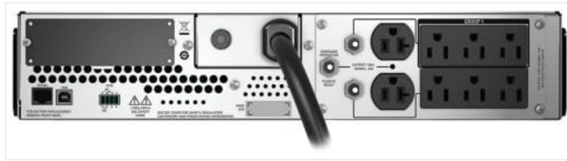
Figure 2: Rear view of the APC SMT2200RM2U Smart-UPS. This image displays the back of the UPS, showing various power outlets (NEMA 5-15R and NEMA 5-20R), an input power cord, communication ports (USB, Serial), and a SmartSlot for expansion cards. Overload protectors are also visible.
