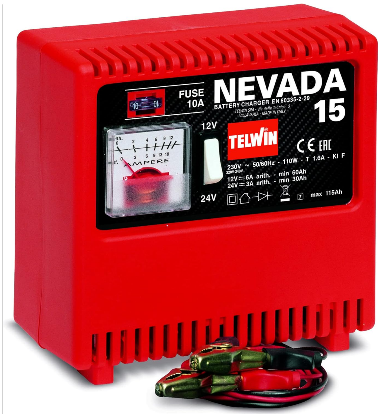
Figure 1: Front view of the Telwin Nevada 15 Battery Charger. The front panel displays the 10A fuse, an ammeter indicating charging current, a voltage selector switch (12V/24V), and printed specifications including input voltage (230V~50/60Hz), absorbed power (110W), and charging parameters for 12V and 24V batteries. The charging clamps are visible at the bottom.
