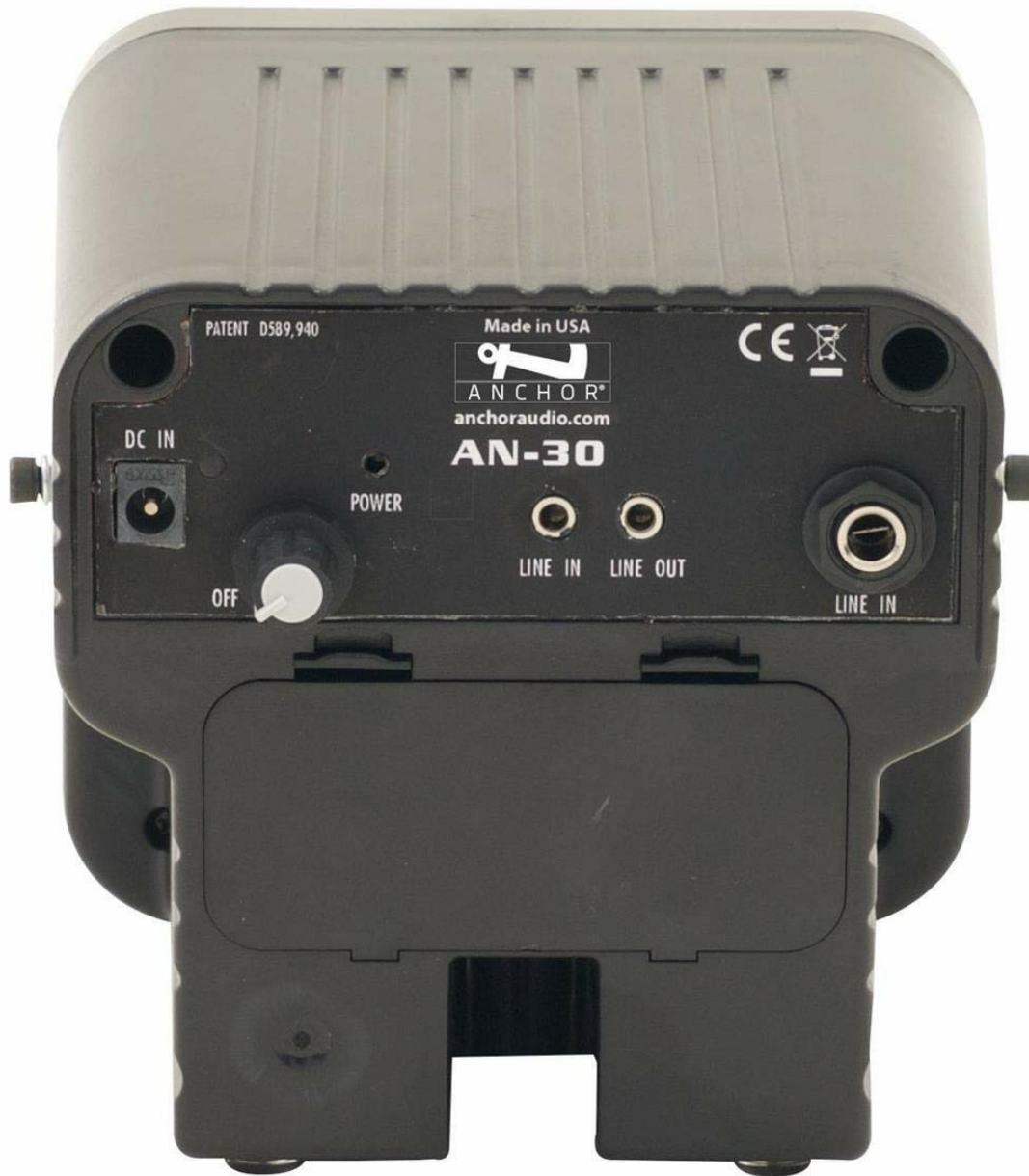
Figure 2.1: Rear panel of the AN-30, illustrating the various input and output connections.
