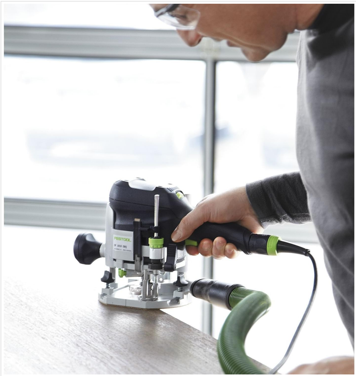
Figure 2: A user demonstrating the Festool OF 1010 EBQ-Plus Router in operation, performing an edge routing task on a wooden surface. The integrated dust extraction hose is visible, connected to the router.
