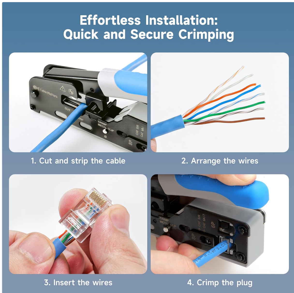
Figure 6: Step-by-step visual guide for RJ45 plug installation.
