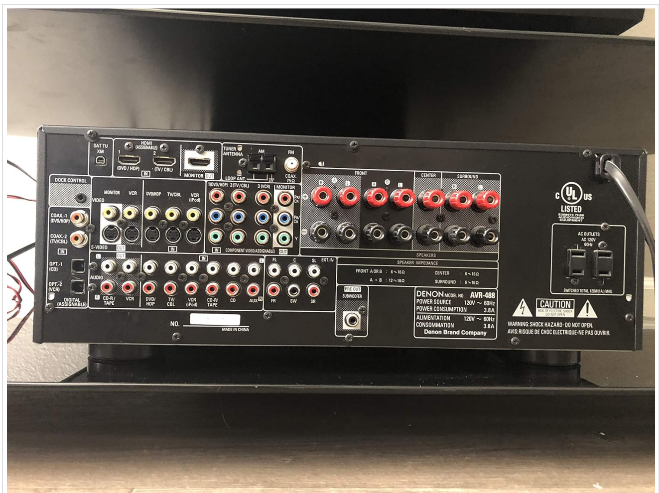
Figure 2.3.1: Rear Panel of Denon AVR-488. This image illustrates the rear panel of the Denon AVR-488 receiver, detailing the extensive array of connectivity options including HDMI, component video, composite video, optical and coaxial digital audio inputs, analog audio inputs, speaker terminals for 5.1 channels, and antenna connections.
