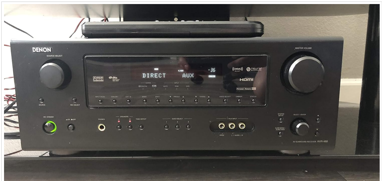
Figure 2.2.1: Front Panel of Denon AVR-488. This image displays the front of the Denon AVR-488 receiver, showing the main display, input selectors, volume knob, and various control buttons for source selection, tone control, and system setup. The power button is located on the lower left.
