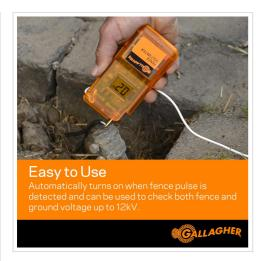
This image illustrates the process of taking a voltage reading with the Gallagher Digital Volt Meter. A hand holds the device, with its top probe touching the electric fence wire and the integrated ground rod inserted into the earth. The digital display shows a reading of "2.0 kV", indicating the fence voltage.
