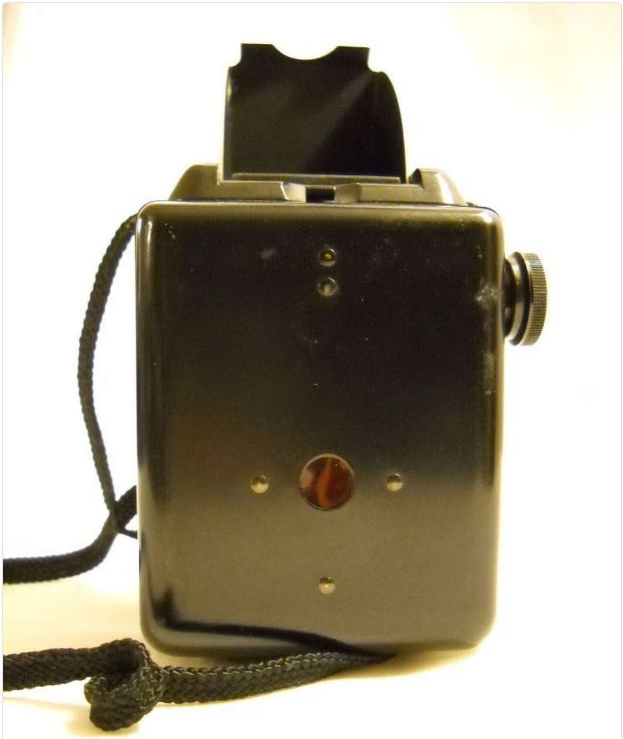
The rear view of the Argus Seventy-Five camera, illustrating the film advance knob on the right side and the small red window used to view film frame numbers. A wrist strap is also visible.
