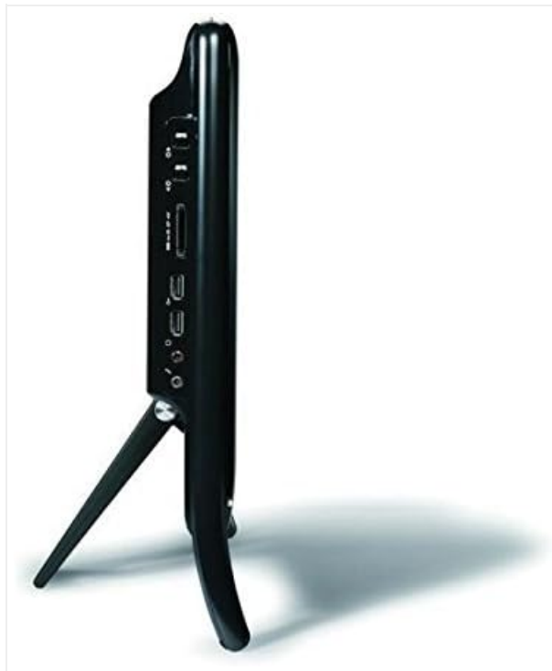
Figure 4.2: Side view of the Acer e-Machines EZ1711 Desktop PC. This image highlights the right side of the computer, revealing several input/output ports and control buttons. These typically include USB ports, audio jacks, and potentially a media card reader or optical drive slot.
