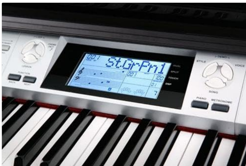
Figure 5: Control panel with Dual and Split buttons
