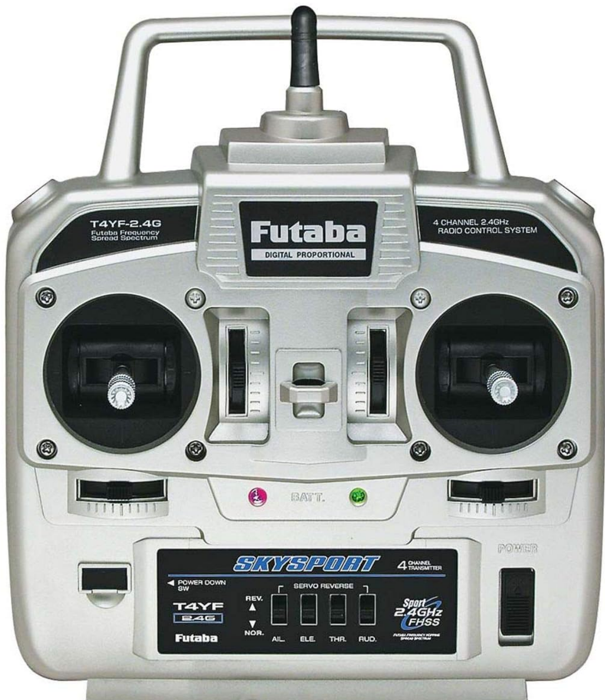
Figure 1: Front view of the Futaba 4YF 4-Channel 2.4GHz FHSS Transmitter. This image displays the main controls including the two joysticks, trim levers, servo reverse switches, power switch, and battery indicator LEDs.
