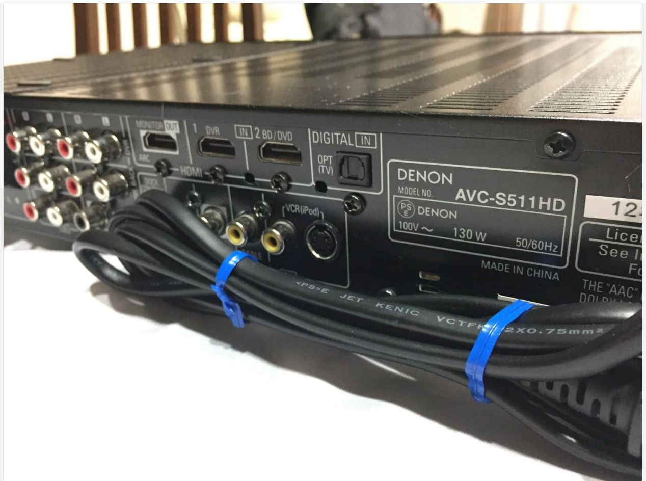
Image 4.1: Rear panel of the Denon AVC-S511HD-K, showing HDMI input/output ports, digital audio inputs, and analog audio/video connections.
