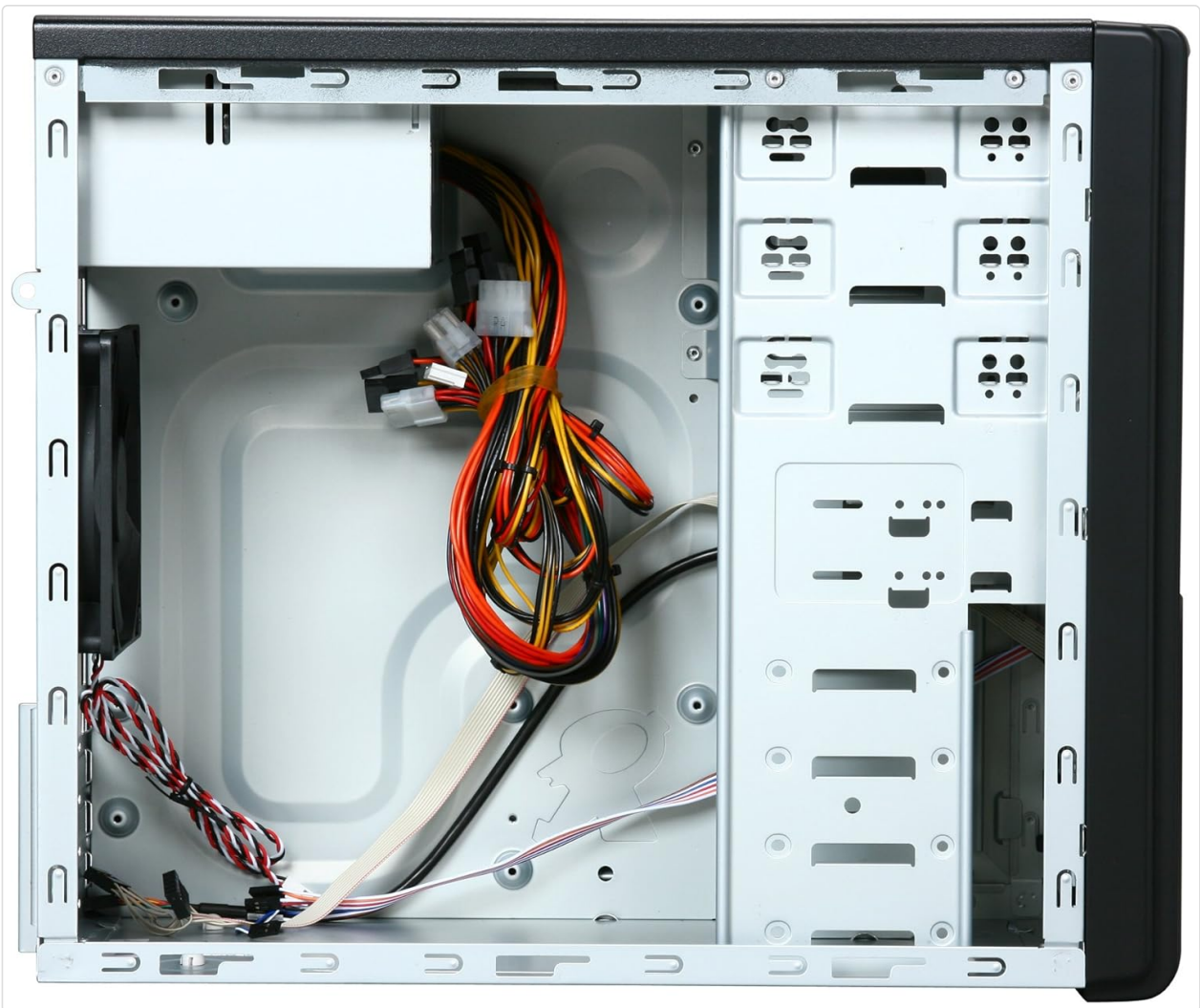
Image 3.2: A closer look at the internal drive bays and the pre-routed power supply cables, illustrating the available space for component installation.
