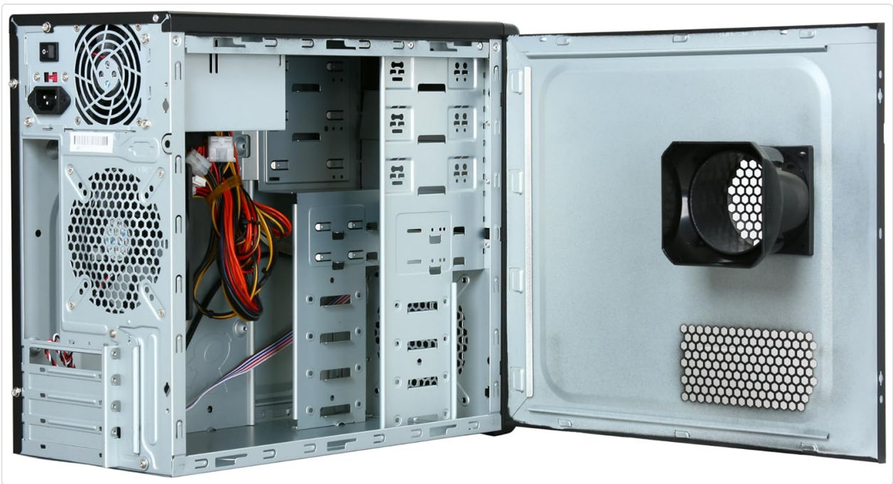
Image 3.1: Interior view of the case with the side panel open, revealing the internal structure, drive bays, and pre-installed power supply.
