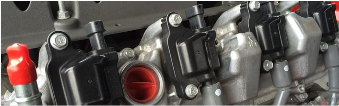
Image: An overhead view of an engine bay, illustrating the typical location of ignition coils which cover the spark plugs.
