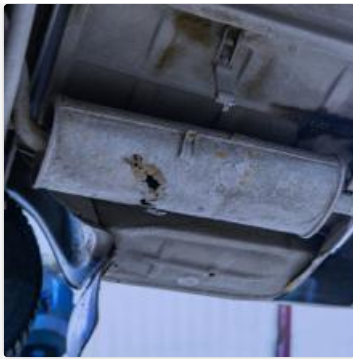
Image: An example of a rusted muffler, illustrating the type of wear that the stainless steel construction of the Quiet-Flow SS muffler is designed to resist.
