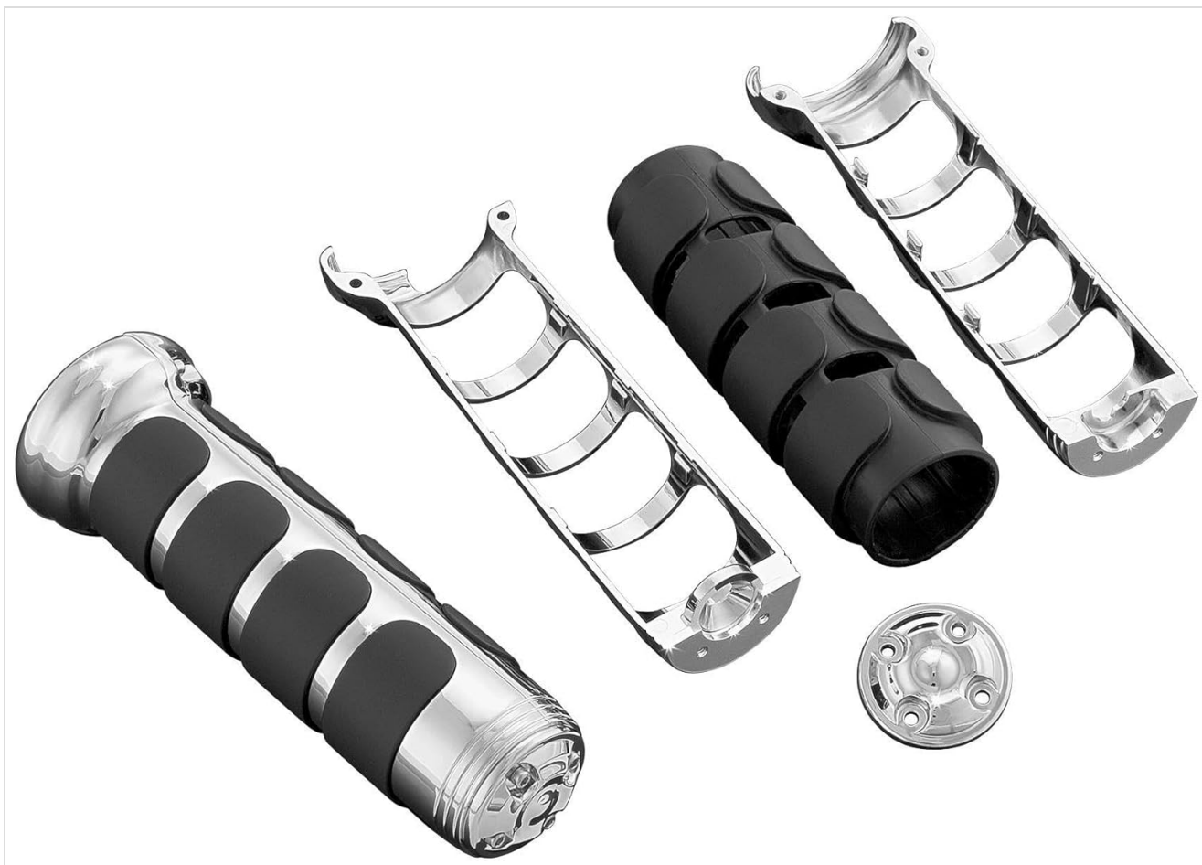
Image: Disassembled Kuryakyn ISO Grips, showing the chrome covers, rubber sleeves, and end cap.
