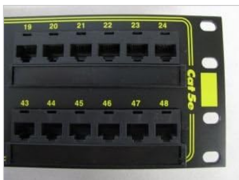
Figure 4.1: Front view of the patch panel, displaying RJ45 ports and numbering.
