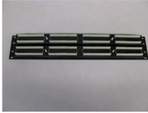
Figure 4.3: Rear view of the patch panel, illustrating the 110 punchdown termination blocks.
