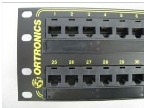
Figure 4.1: Front view of the patch panel, displaying RJ45 ports and numbering.
