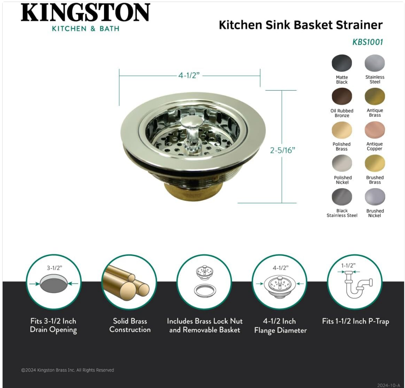
Figure 1: Product Diagram and Dimensions. This image illustrates the key dimensions and components of the sink basket strainer, including its compatibility with a 3-1/2 inch drain opening, solid brass construction, included lock nut and removable basket, and overall flange diameter and depth.
