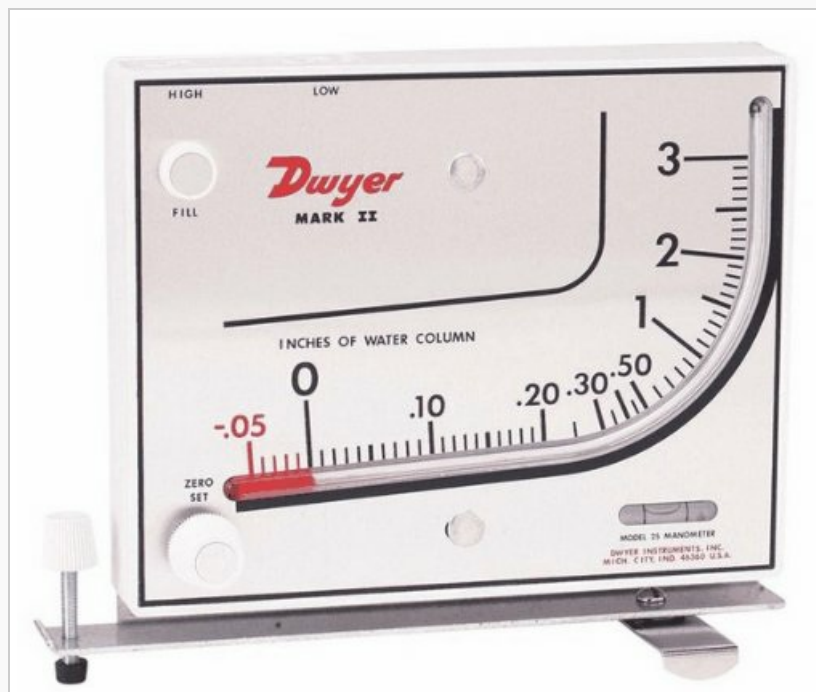
Figure 1: Front view of the Dwyer Mark II Model 25 Inclined Manometer. The image displays the instrument's face with a scale marked in inches of water column, ranging from -0.05 to 3 inches. Key features visible include the "HIGH" and "LOW" pressure ports, a "FILL" port, a "ZERO SET" knob, and the Dwyer Mark II branding. A spirit level is integrated at the bottom right for proper leveling during operation.
