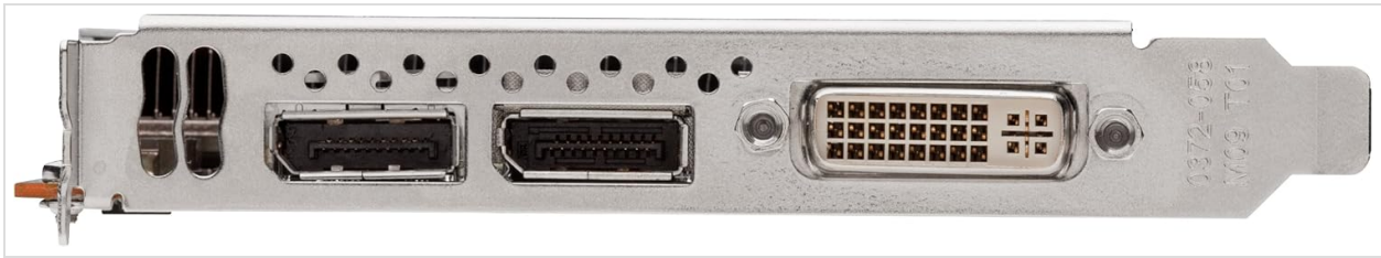
Image: A close-up view of the rear bracket of the PNY NVIDIA Quadro 2000, clearly showing the two DisplayPort connectors and one DVI-I connector.
