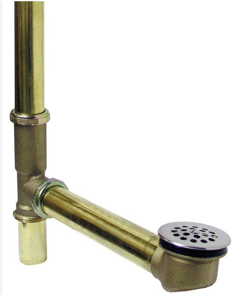
Figure 1: Watts 98CP Trip Lever Bath Drain assembly. This image displays the complete drain unit, including the chrome-finished trip lever overflow plate, the brass overflow tube, the brass T-fitting, the brass waste shoe, and the chrome-finished drain stopper.
