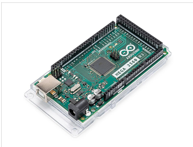
Figure 1: Angled view of the Arduino Mega 2560 REV3 board, showcasing its various pins and USB port.
