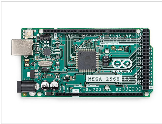
Figure 2: Top-down view of the Arduino Mega 2560 REV3 board, highlighting the ATmega2560 microcontroller and pin labels.
