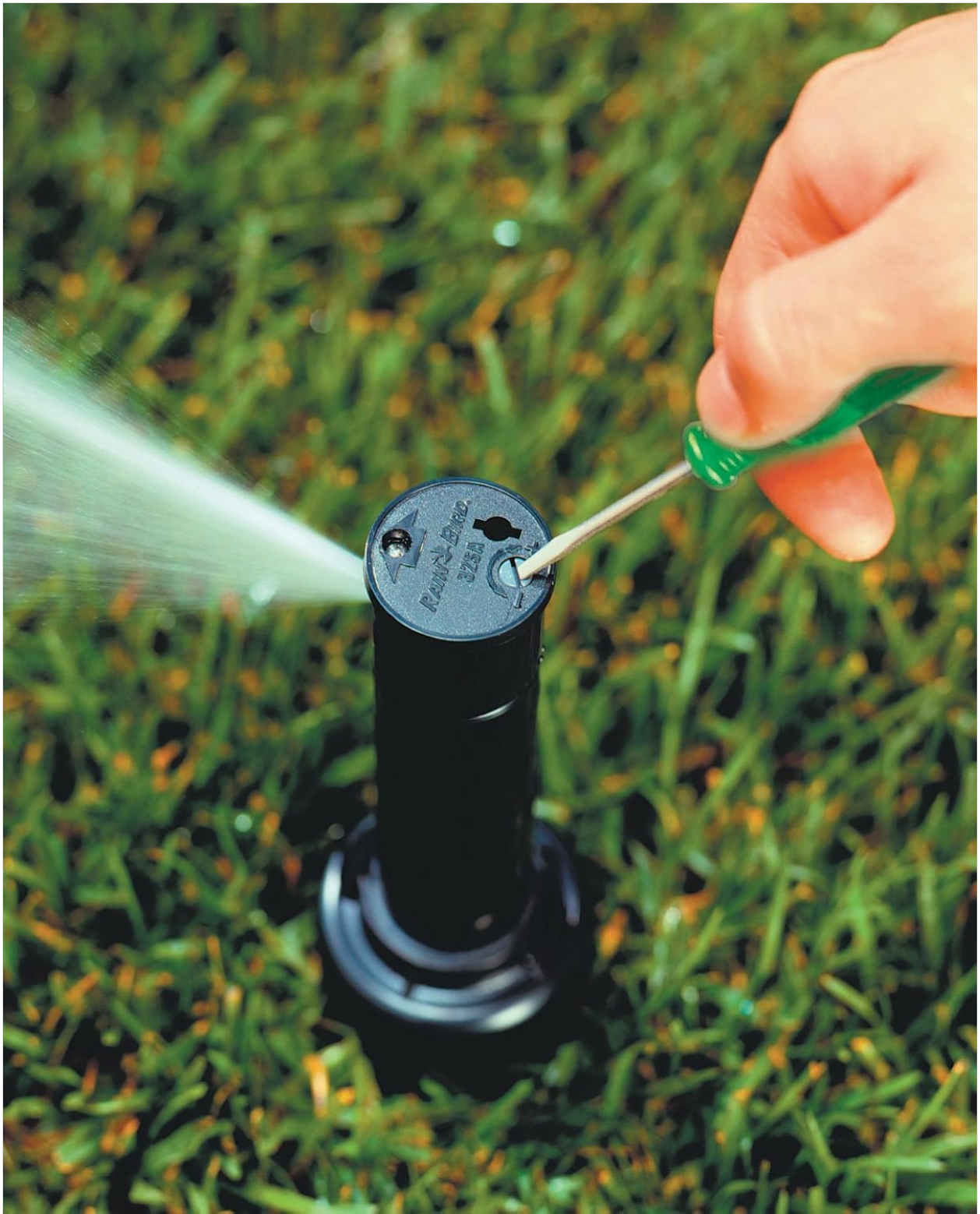
Figure 5: Adjusting Spray Pattern
