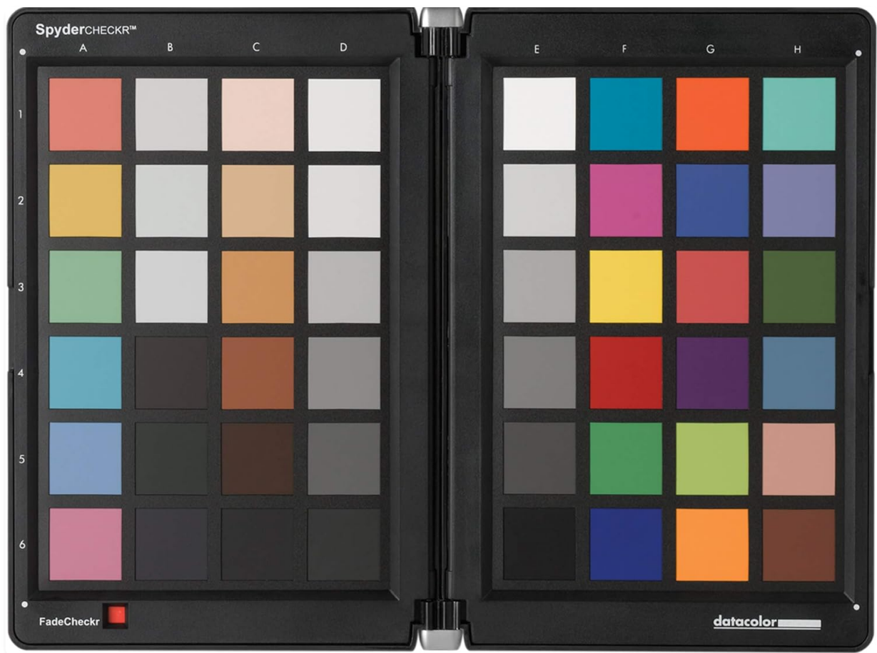
Image 1.1: The Datacolor Spyder Checkr opened, revealing its 48 color patches and grey scale for calibration.
