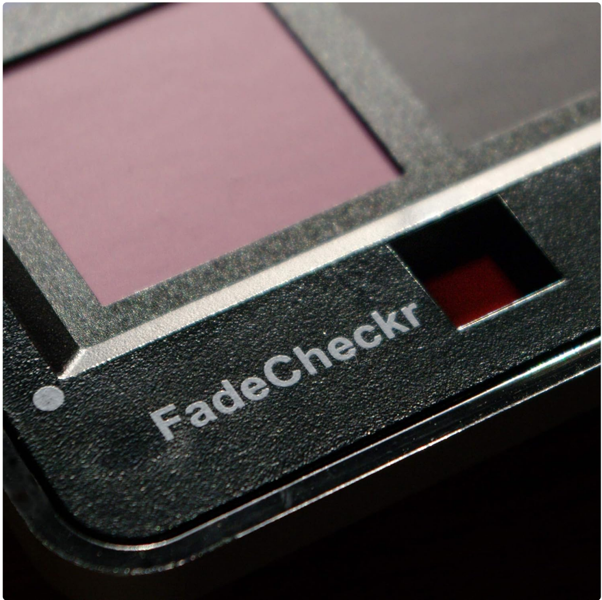
Image 2.1: Detail of the Fade Checker patch, indicating the condition of the color targets.
