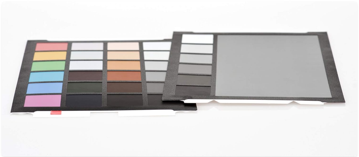
Image 5.2: The individual color target cards removed from the Spyder Checkr casing.
