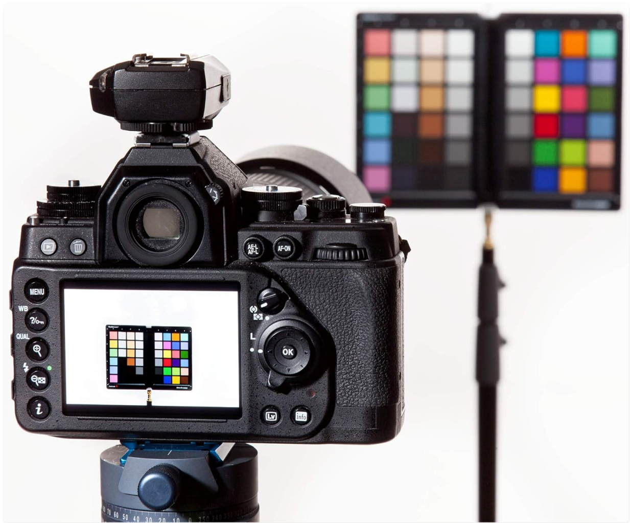
Image 3.1: A camera positioned to capture the Spyder Check for color calibration.
