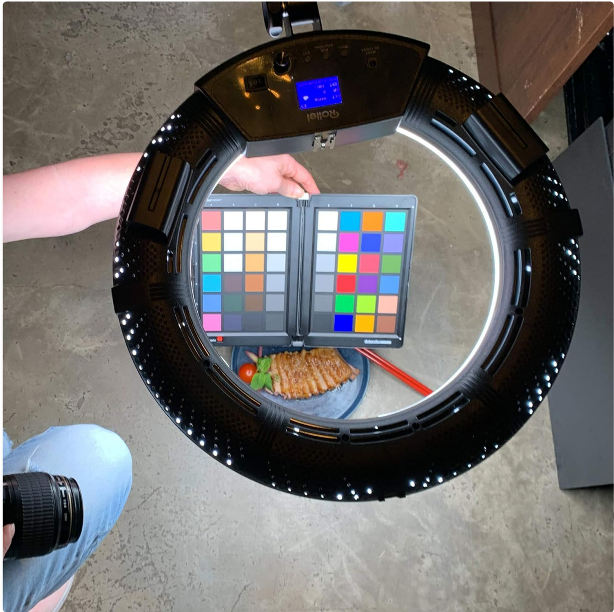
Image 4.2: The Spyder Checkr placed within a setup, illuminated by a ring light for consistent color capture.
