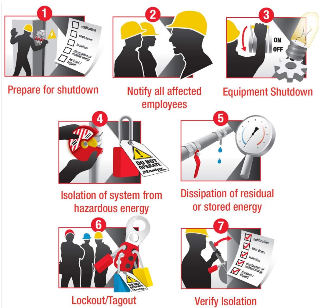
Image 5.2: A visual representation of the seven essential steps in a Lockout/Tagout procedure, from preparation to verification of isolation.
