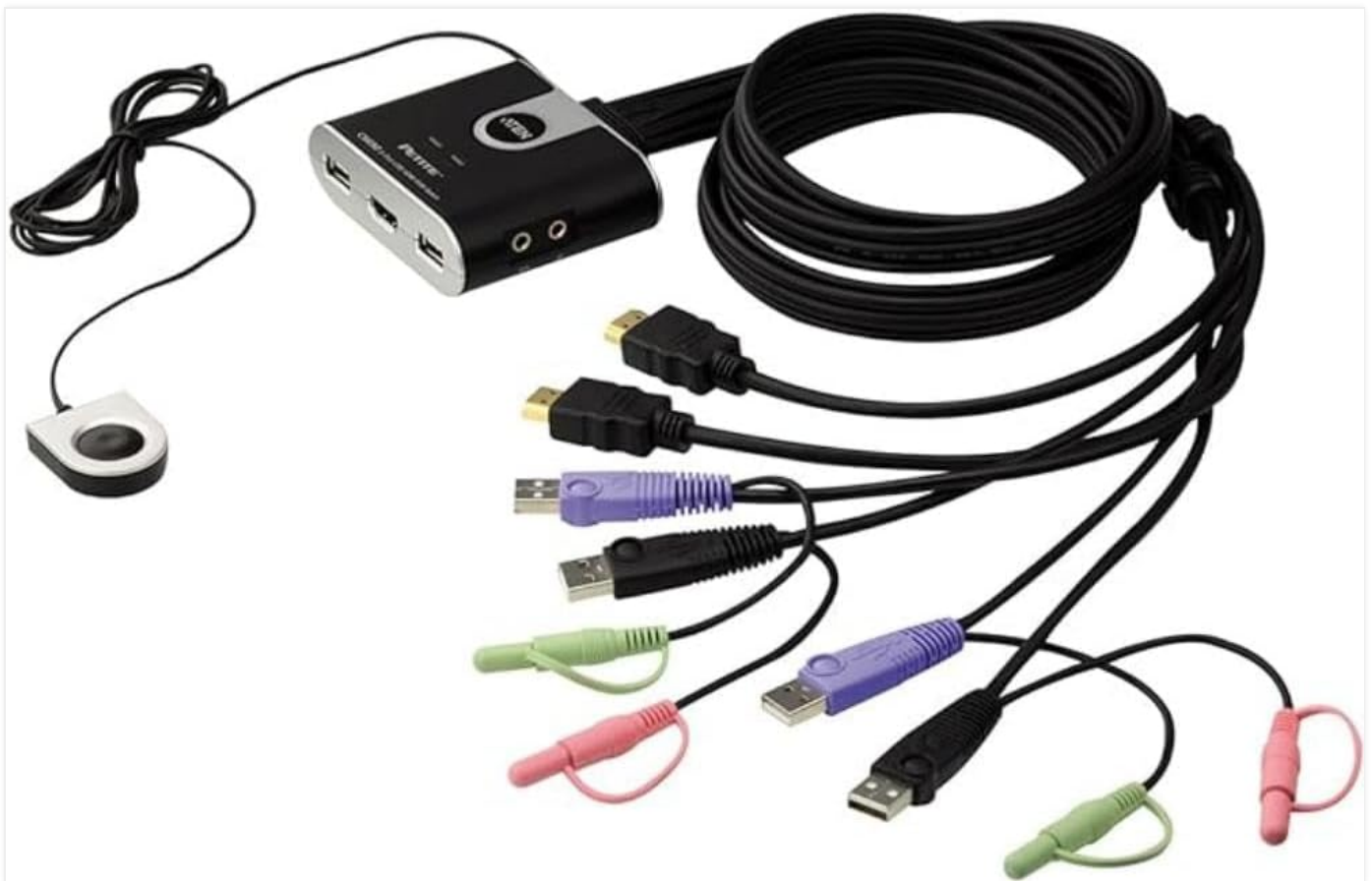
Figure 3: ATEN CS692 KVM Switch with Cables. This image displays the compact KVM unit, its integrated HDMI, USB, and audio cables for connecting to two computers, and the separate remote port selector for easy switching.
