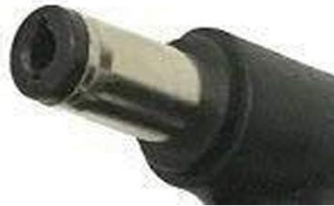
Figure 4.1: Barrel Connector. This image shows a close-up of the DC barrel connector, which plugs into the compatible electronic device.
