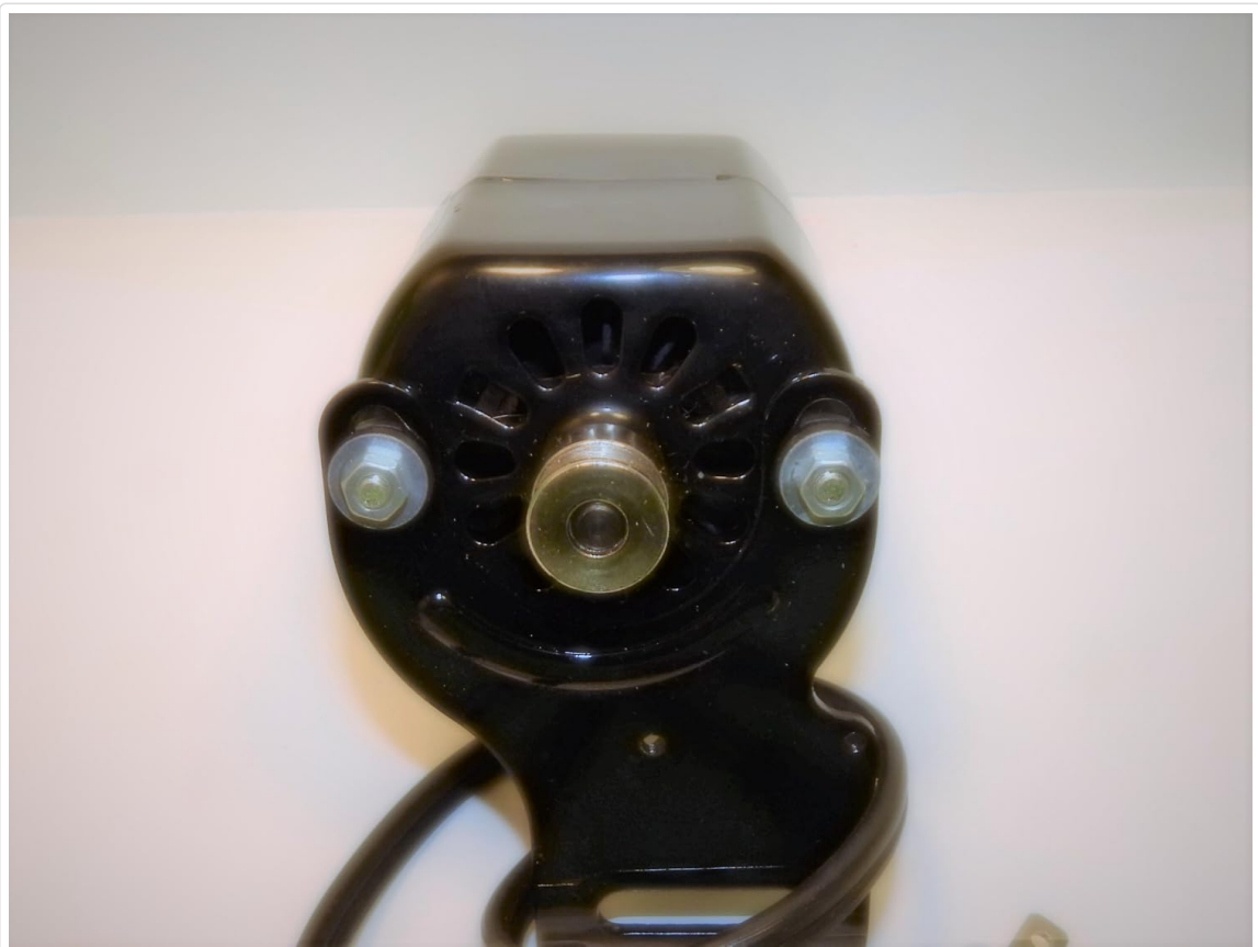
Image: Front view of the Alphasew motor, displaying the pulley for belt attachment.
