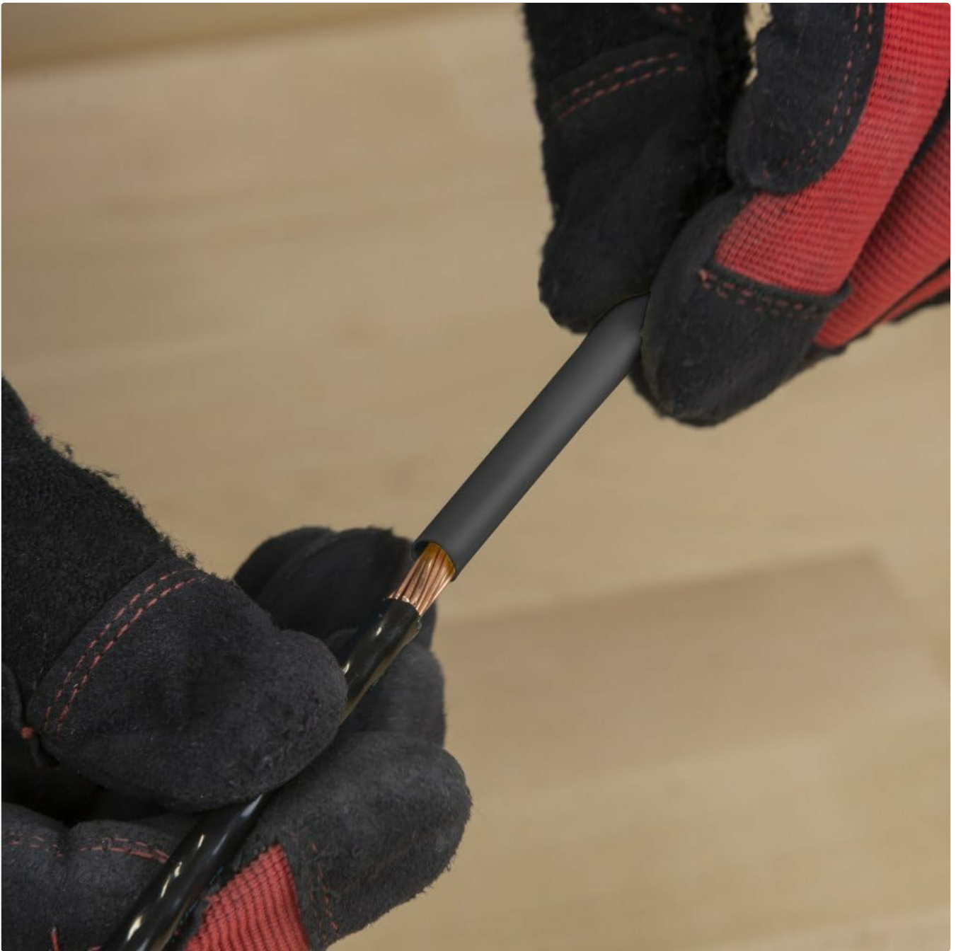
Figure 3: Sliding heat shrink tubing onto a prepared wire.
