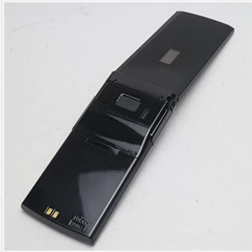
Figure 2: Rear view of the F-10B, indicating the location for battery and SIM card insertion.
