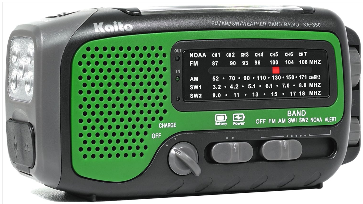
Figure 3: Front panel controls including tuning dial, band selector, and volume.
