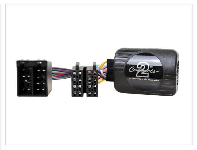
This image displays the Connects2 CTSCT002 module, a black rectangular unit with the 'Connects2' logo, connected to two multi-pin ISO wiring harnesses. These harnesses are designed to integrate with a vehicle's existing wiring and an aftermarket car stereo.
