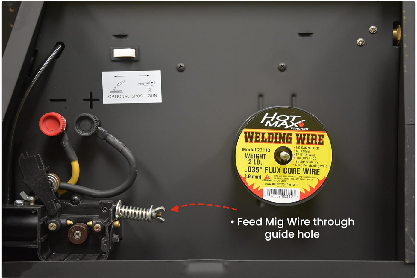
Figure 1: Internal view of the welder with the wire feed mechanism. Ensure the welding wire is fed correctly through the guide hole and into the drive roller system.
