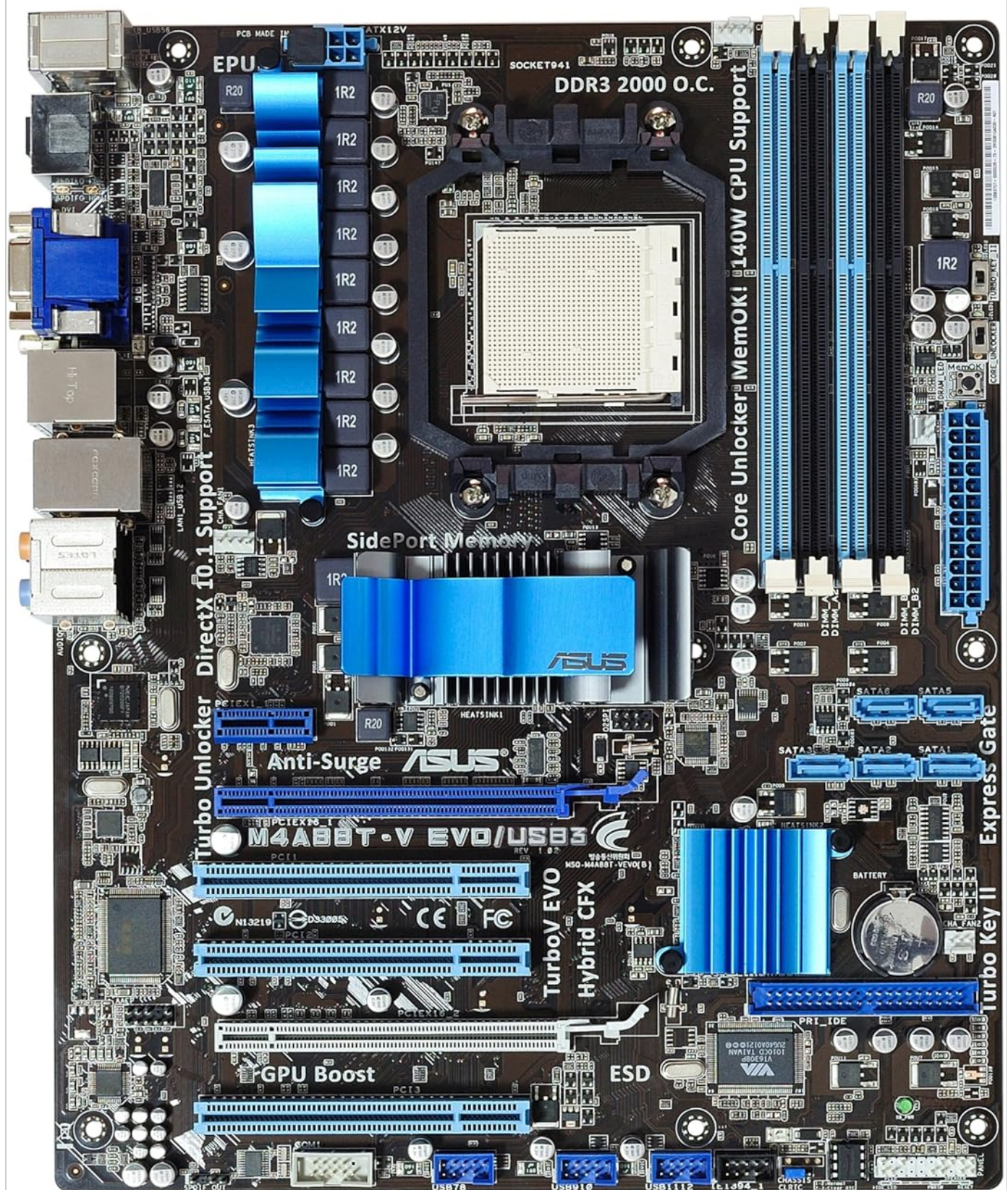
Figure 1: Top-down view of the ASUS M4A88T-V EVO/USB3 Motherboard, highlighting the CPU socket, RAM slots, and various expansion slots.
