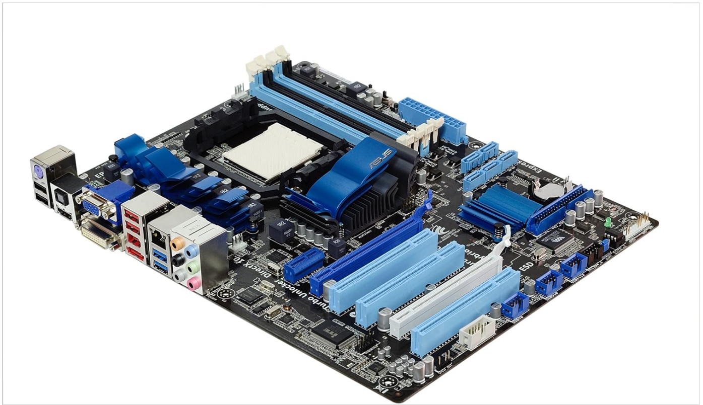
Figure 3: An angled view of the motherboard, showcasing the rear I/O panel, expansion slots, and memory DIMM slots.
