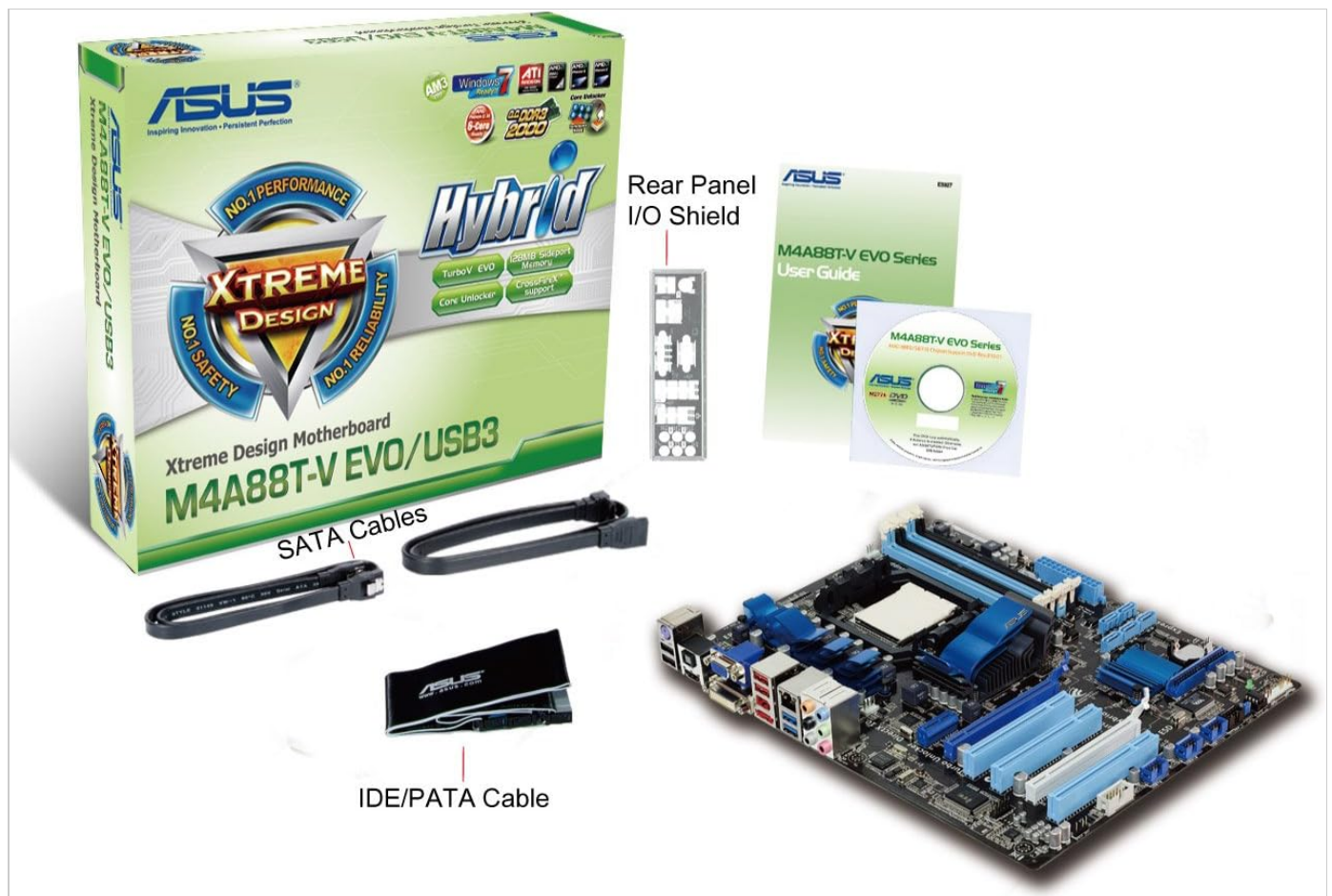
Figure 2: The ASUS M4A88T-V EVO/USB3 Motherboard with its standard accessories, including SATA cables, an IDE cable, the I/O shield, and documentation.
