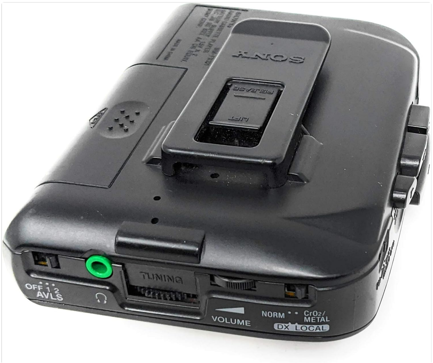
Figure 2: Side and rear view of the Sony Walkman WM-FX101. This perspective highlights the side controls such as volume, tuning, AVLS switch, headphone jack, and the rear belt clip.
